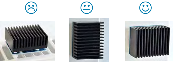
Heat sink orientation matters!
