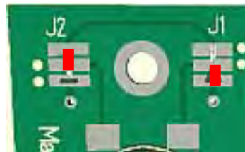
Solder pads J_1 and J_2 connection for reversed heat flux direction
