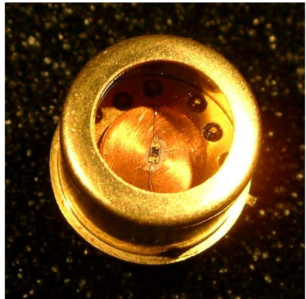
Fig. 6: VCSEL mounted on MicroPelt ® Peltier cooler in TO8 housing
