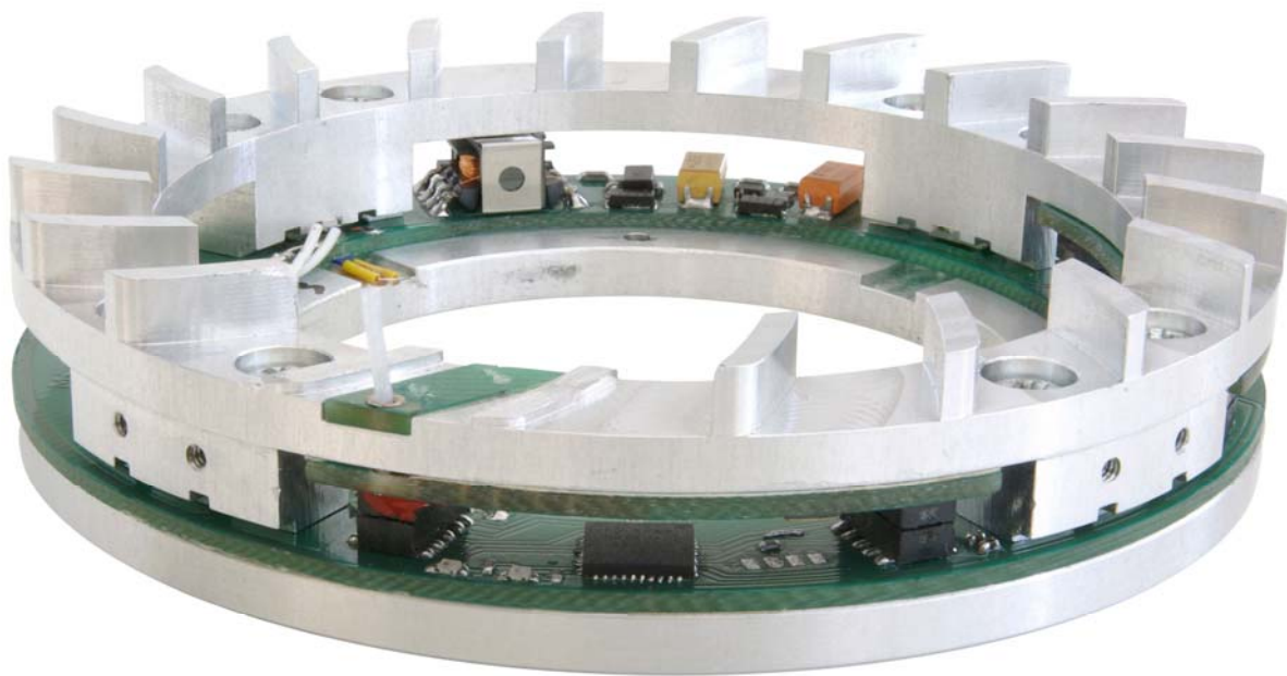
TE-Power RING with integrated radio module
