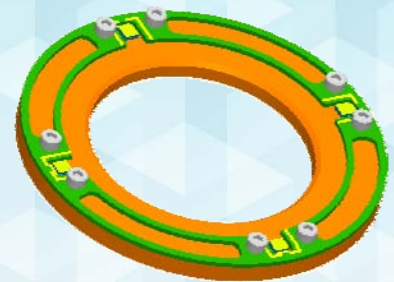
Thermogenerator-based wireless sensor for bearing monitoring
