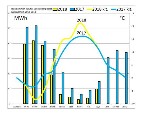
Energy consumption of Leppäkoski office building in the past year 2018 compared to 2017. MWh Energy on the left scale. Average temperatures marked with lines and ° C scale on the right.
