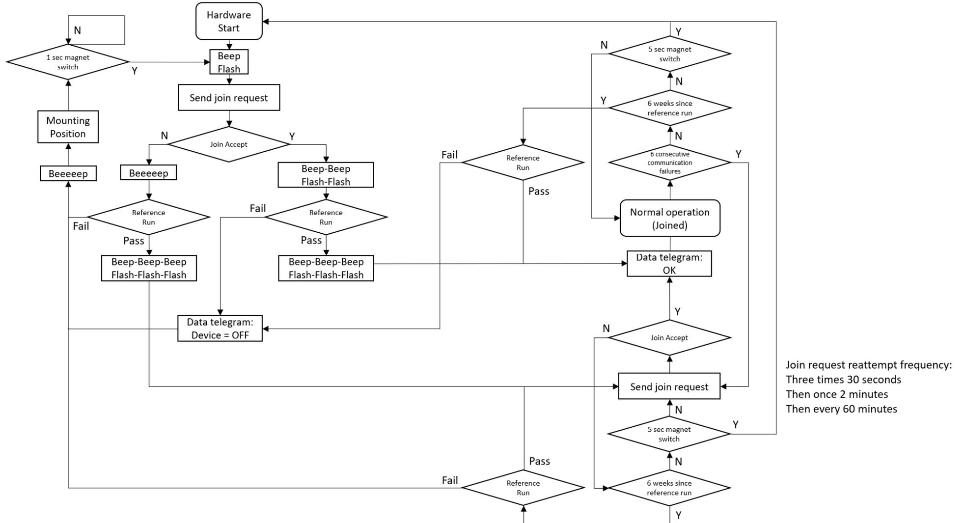
The unit has no user-accessible buttons to avoid manipulation of the device in public environments. Installers rely on a pen-shaped magnet to perform tasks related to the installation.
