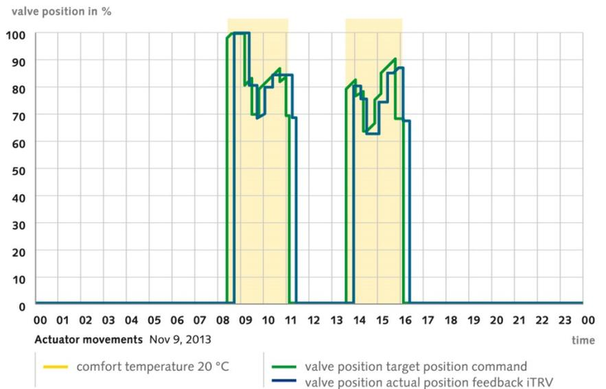
In summary, the field test shows that the energy-autonomous thermostatic radiator valve performs reliably even under the most stringent conditions—a relatively low and fluctuating inlet temperature typical for modern heating systems, a well-insulated house and the relatively warm outdoor temperatures in the transitional autumn months—and is fully equal to the battery-driven valves when it comes to convenient control.
