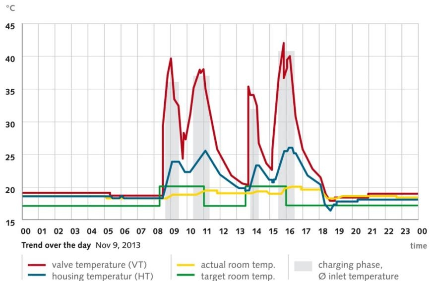
**Energy-autonomous valve handles up to 40 actuating movements per day**
